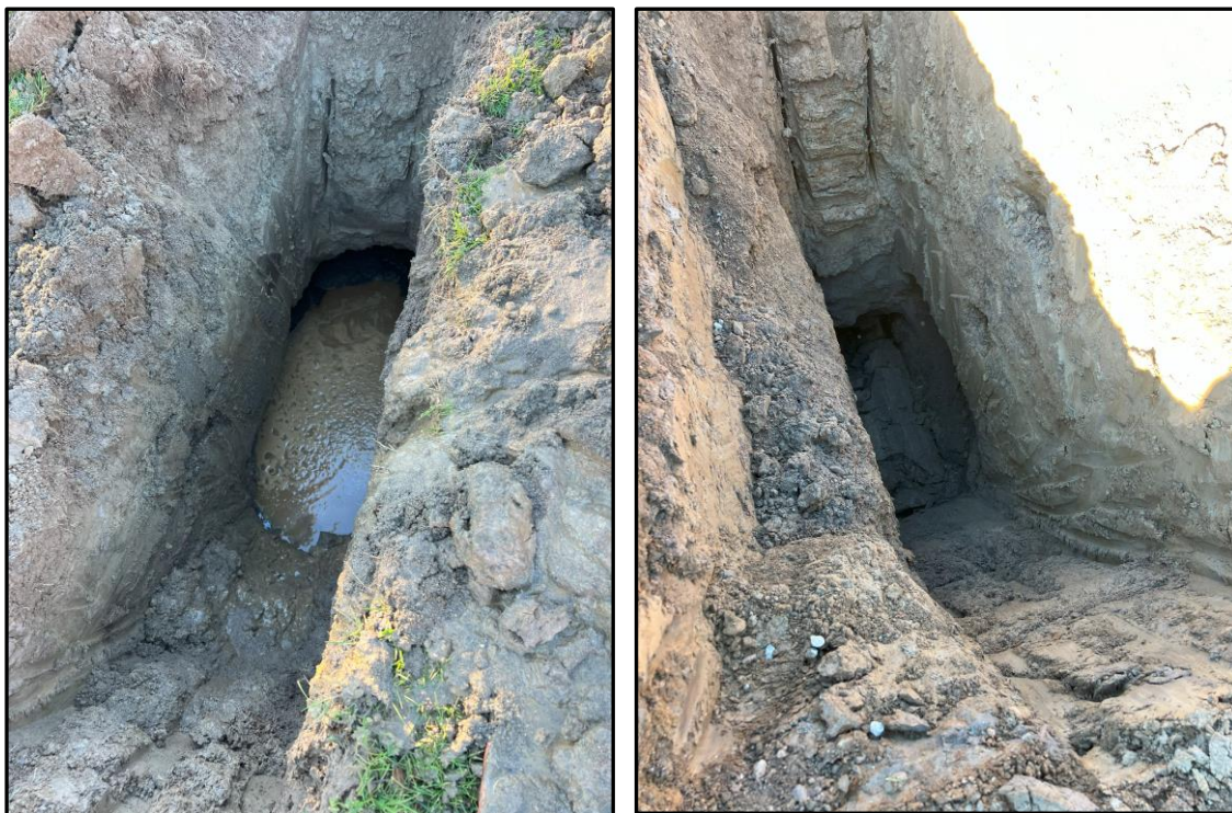
Images 3 and 4. TP-1 with groundwater at 4 feet BGS (left) and TP-2 (right) during explorations. Photos were taken during the site explorations on February 16 th , 2024.
